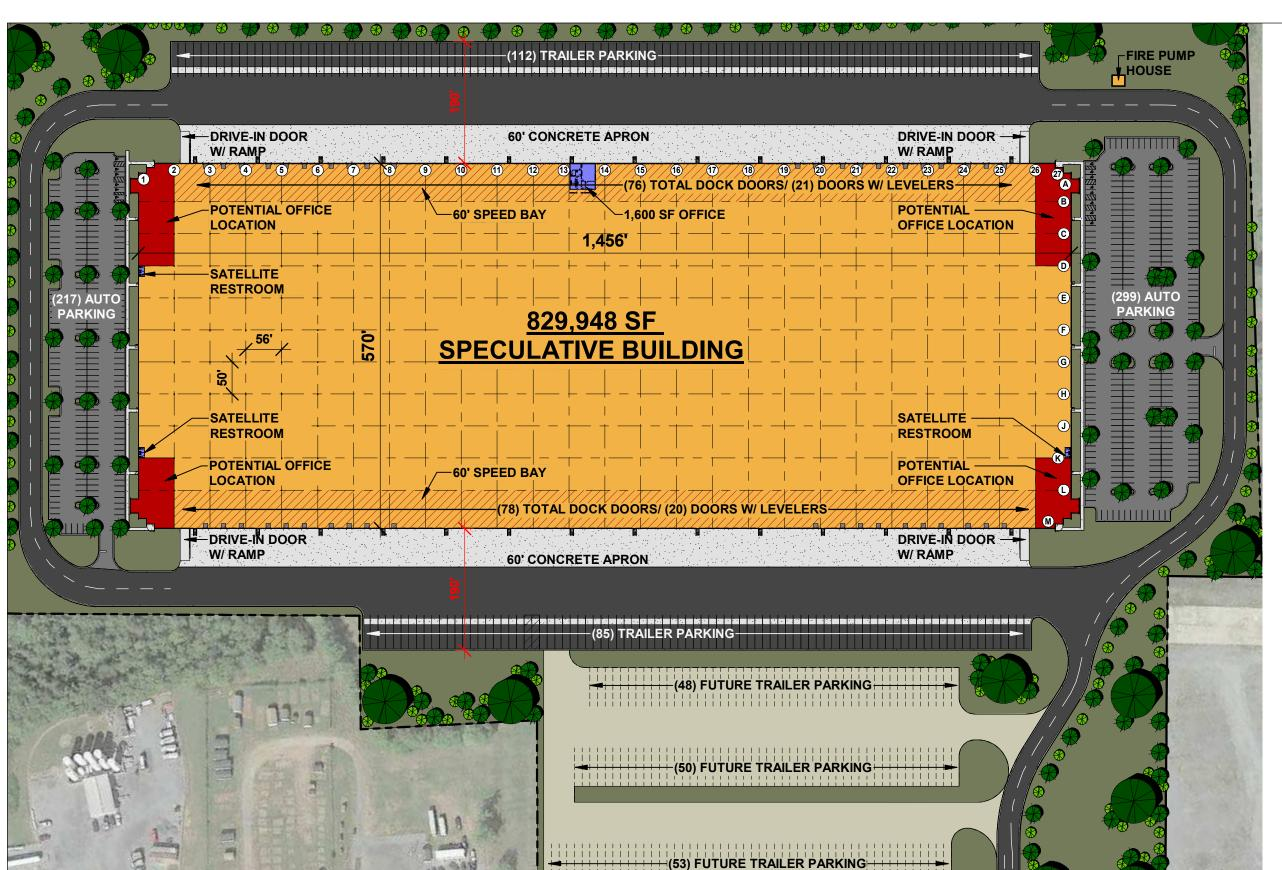
**NOTES CAR PARKING** PLAN EAST 299 217 PLAN WEST TOTAL 516 **TRAILER PARKING** PLAN NORTH 112 PLAN SOUTH 85 **TOTAL** 197 **FUTURE SPACES** 151 \*TRAILER PARKING SIZED AT 12' WIDE X 60' DEEP **DOCK DOORS PLAN NORTH W/OUT LEVELERS 55** PLAN NORTH W/ LEVELERS 21 PLAN SOUTH W/OUT LEVELERS 58 PLAN SOUTH W/ LEVELERS 20 **TOTAL** 154 **WAREHOUSE LIGHTING** 25 FOOT CANDLES
